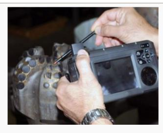
With Shell's virtual presence system, a rig worker can use a camera to explain a problem with a drill bit.
