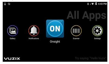
**Step 4:** Enable voice recognition. You must enable voice recognition in order for the Vuzix device to execute recognizable voice commands. To enable voice recognition say "**HELLO VUZIX**".
