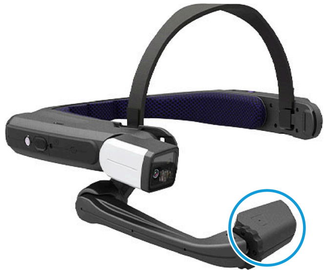
Figure 3-3 Adjusting the Display Pod
